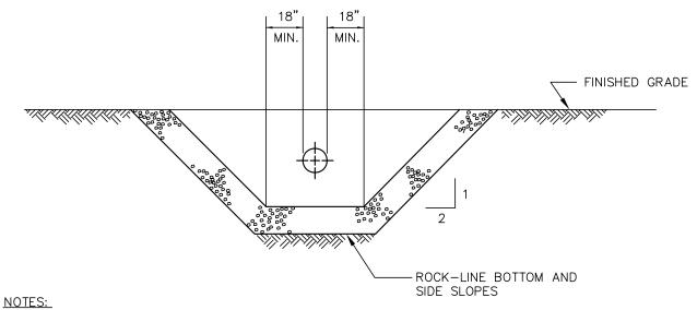
1. PLACE QUARRY SPALLS IN FRONT OF CULVERT DISCHARGE, ENGINEER SHALL SIZE QUARRY SPALL BERM
