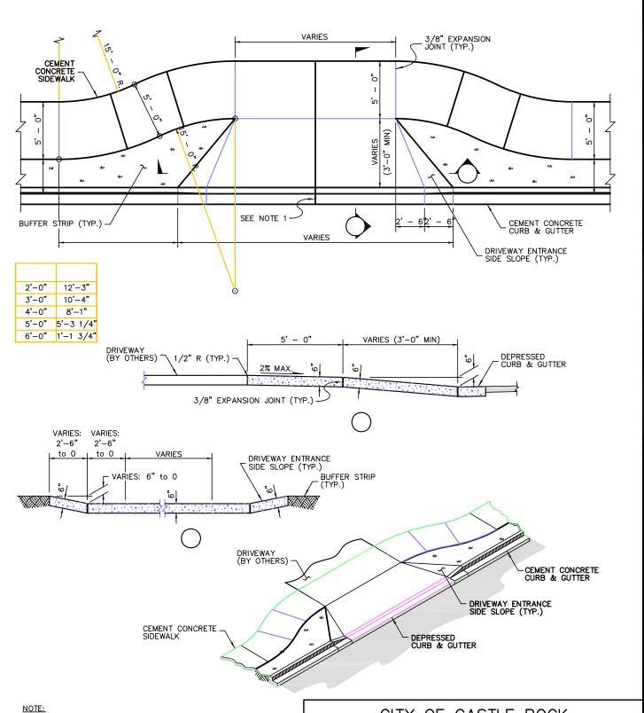
1. WHEN THE DRIVEWAY WIDTH EXCEEDS 15 FEET, CONSTRUCT A FULL DEPTH EXPANSION JOINT WITH 3/8" JOINT FILLER ALONG THE DRIVEWAY CENTERLINE. CONSTRUCT EXPANSION JOINTS PARALLEL WITH THE CENTER-LINE AS REQUIRED AT 15' MAXIMUM SPACING WHEN DRIVEWAY WIDTHS EXCEED 30'.
